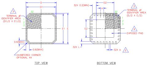
The USB3300 is offered in a compact 32 lead-free QFN package.
