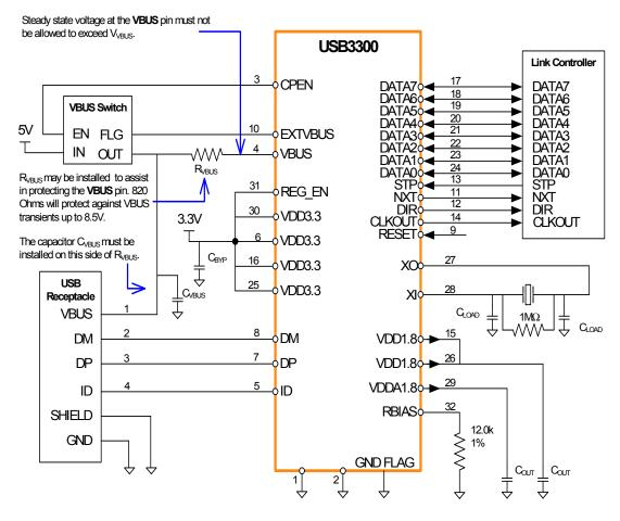
Figure 6 USB3300 Application Diagram (Host or OTG)
