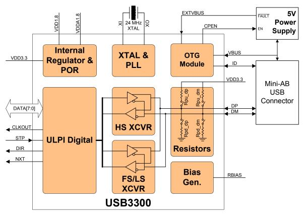
Figure 3 USB3300 Block Diagram
