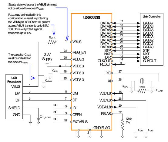
Figure 5 USB3300 Application Diagram (Peripheral)
