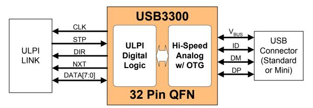
Figure 1 Basic ULPI USB Device Block Diagram
