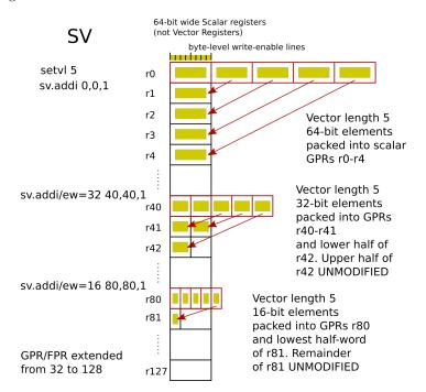
Figure 4: three instructions, same vector length, different element widths
