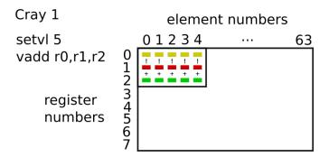
Figure 3: Cray Vector registers: 8 registers, 64 elements each
